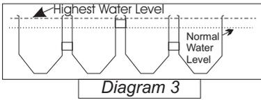
The filter will need to be buried in the ground along side the pond so that the normal water level within the pond is above the top of the lowest outlet but is below the top of the highest baffle. See *diagram 3*
